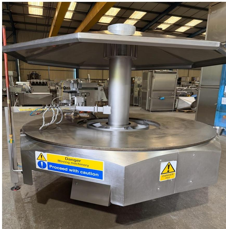
Complete pancake production line featuring two rotating hot plates and a wire belt system that automatically flips pancakes to cook both sides evenly. Built for reliable high-volume production.
