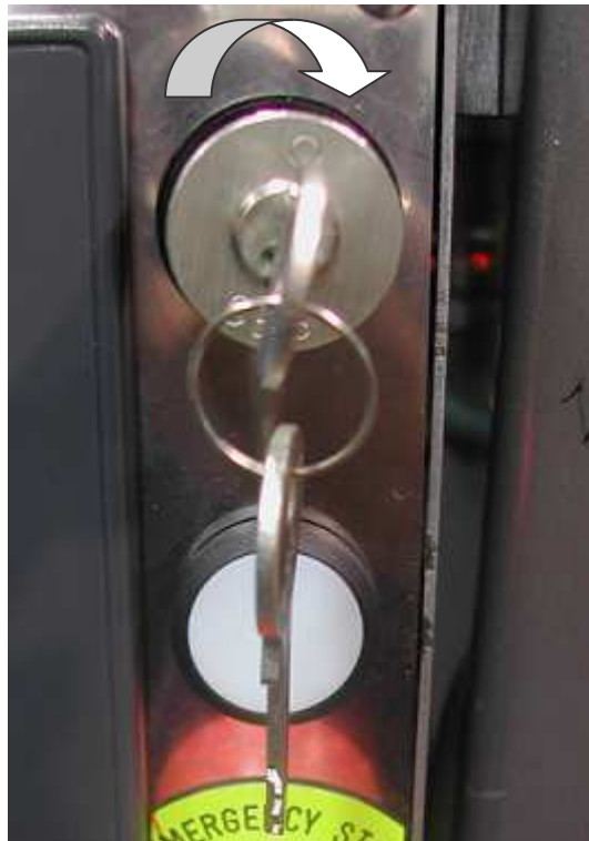
Fig.11.1 Mobile safeguards disabling key
